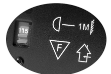
Figure 1 - AC Voltage Switch
